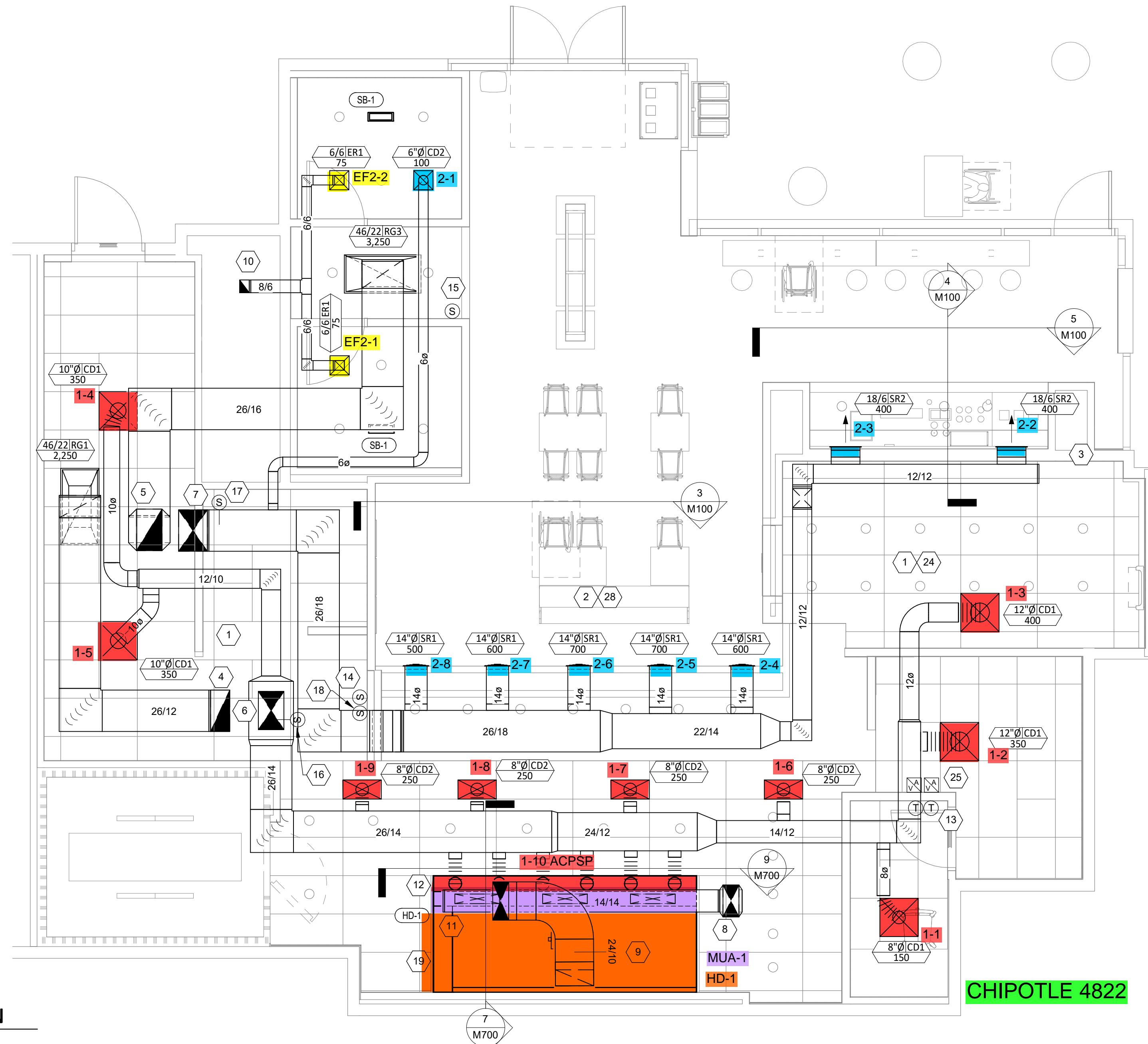
HVAC FLOOR PLAN 1/4" = 1'-0"
