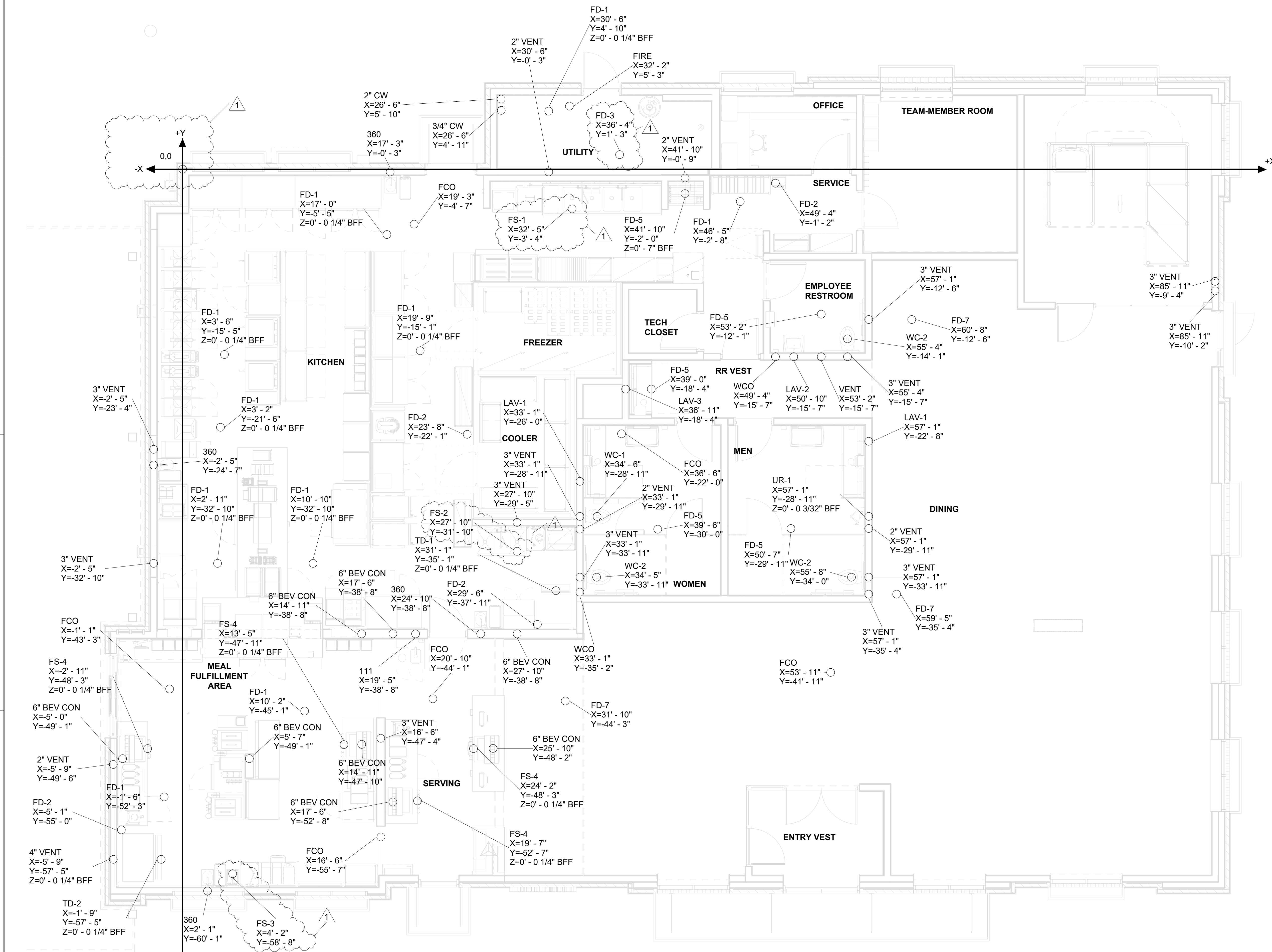
1 SLAB ROUGH-IN PLAN 1/4" = 1'-0"
