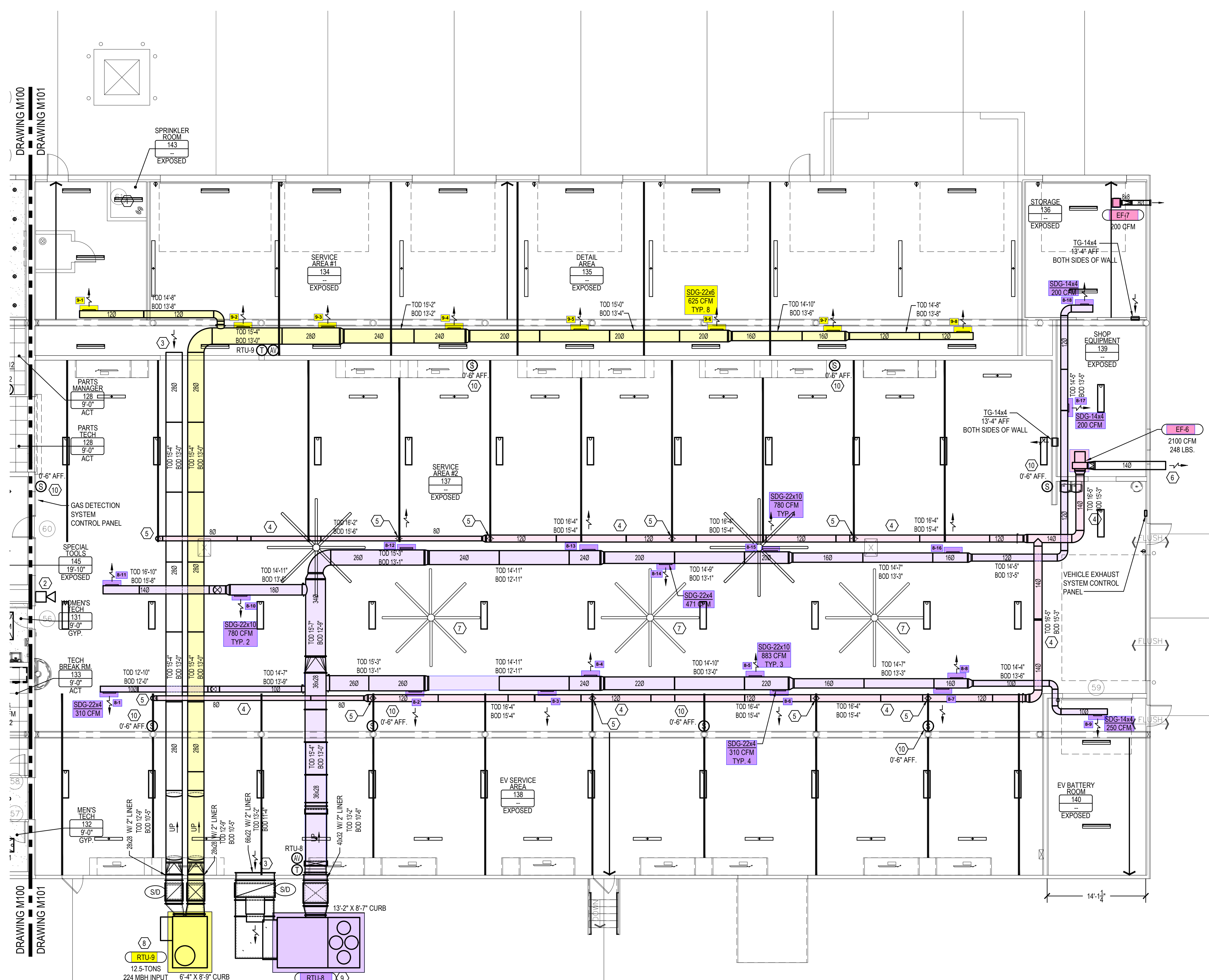
1ST FLOOR SERVICE AREAS HVAC PLAN SCALE: 1/8" = 1'-0"
