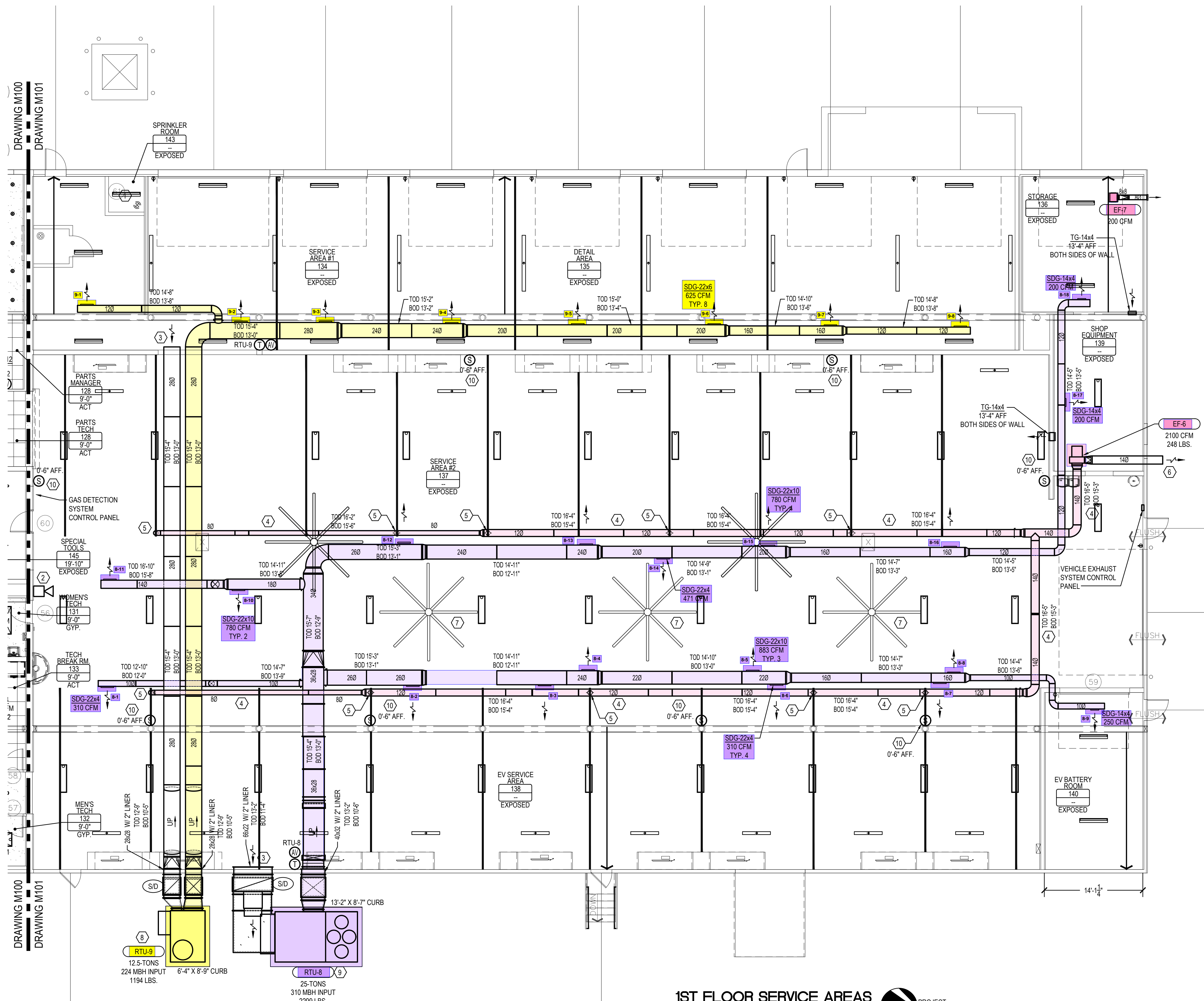
1ST FLOOR SERVICE AREAS HVAC PLAN SCALE: 1/8" = 1'-0"
