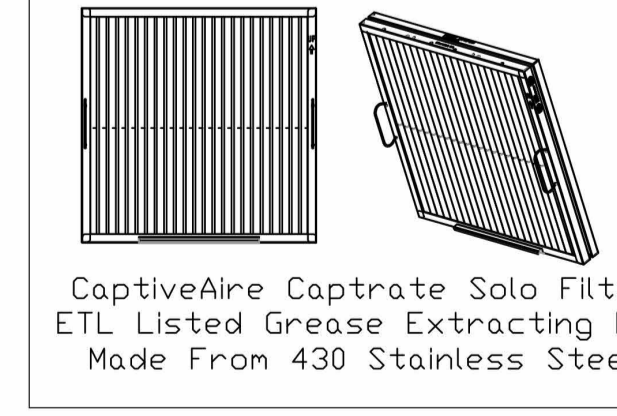
CaptiveAire Captrate Solo Filter ETL Listed Grease Extracting Filter Made From 430 Stainless Steel
