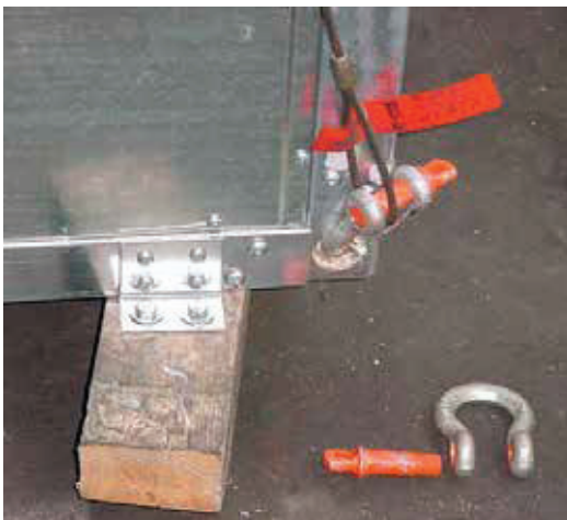
Figure 12 - Correct lifting with shackle with connector corners
