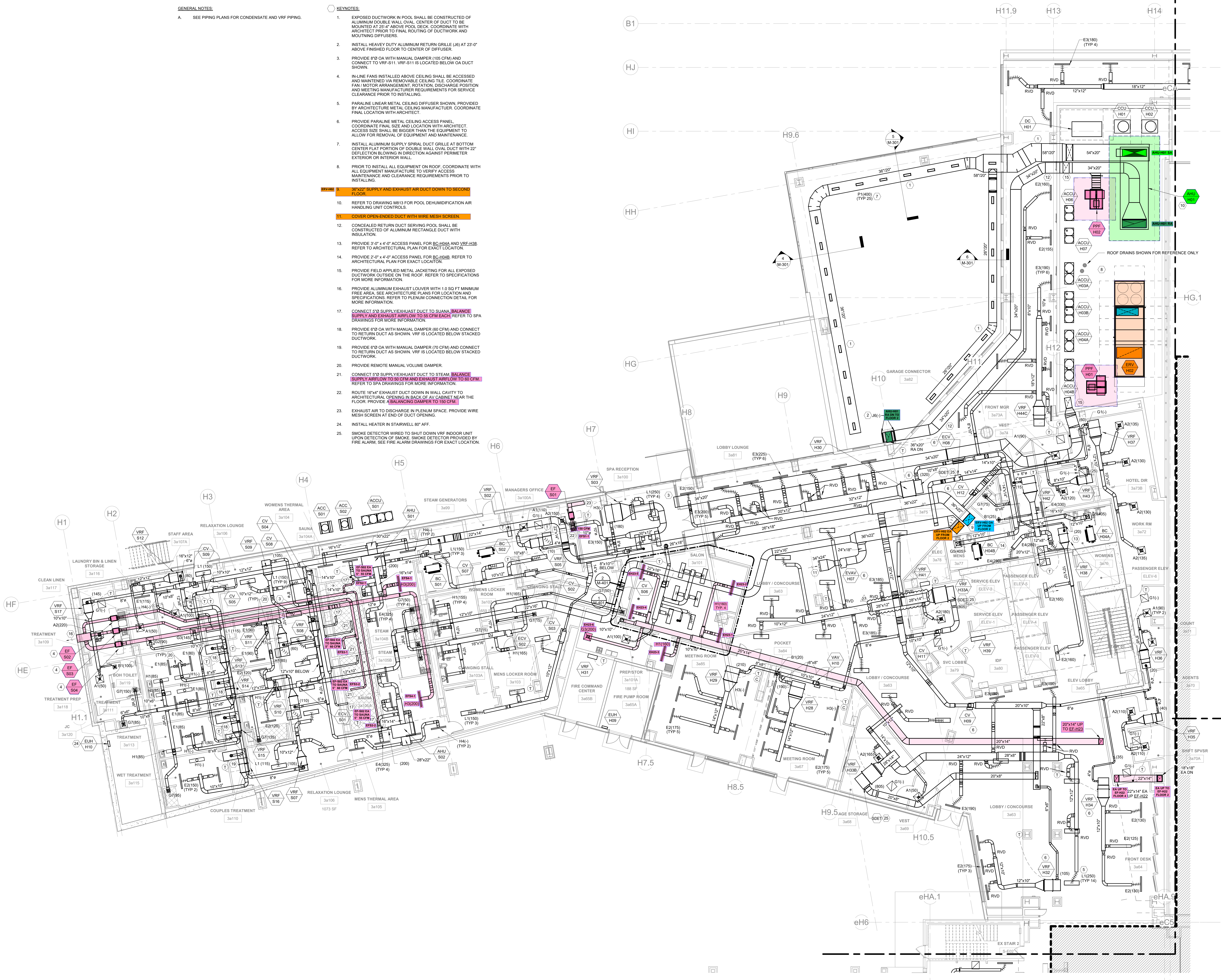
1 HVAC DUCTWORK - THIRD FLOOR LEVEL - AREA A 1/8" = 1'-0"
