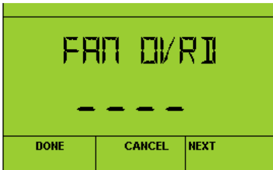
Set fan On/Off [nviFan, state]
