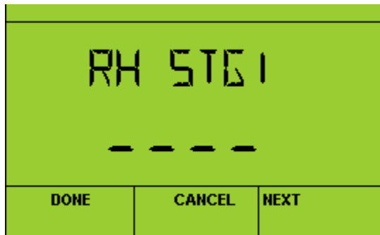
Configure Reheat Stage 1 [nciLogicalOutVav, HtgStg1]
