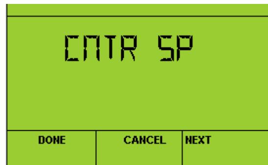
Ignore or use center setpoint (setpoint can still be changed from home screen but will be ignored) [nciWallModCom, UseWmStPt]
