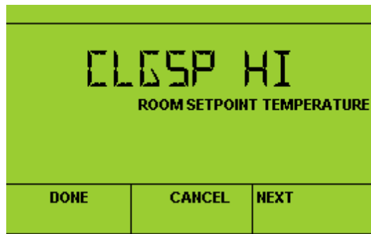
Maximum cooling setpoint [nciWallModCom, MaxClgSetPt]
