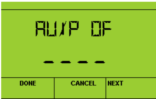
Configure Auxiliary Relay pulse OFF [nciLogicalOutVav, AuxPlsOff]
