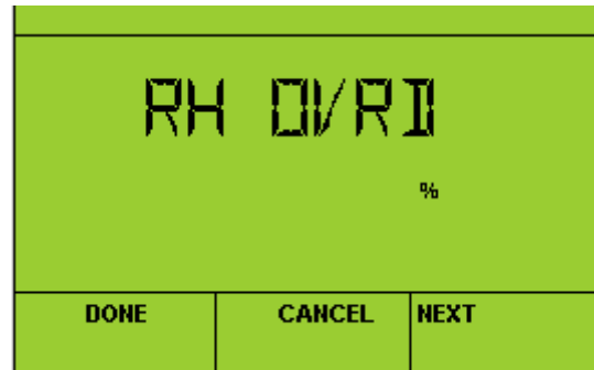
Reheat override as a percent number of stages or modulation [nviValveOvr, reheatPos]
