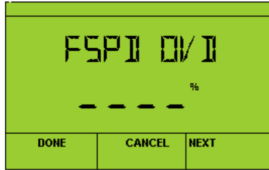
Set modulating Fan Speed [nviFan, value]
