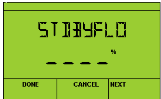
Standby minimum damper position [nciFlowSP, StbyMinFlowPos]
