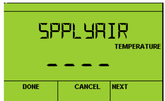
View supply air temperature
