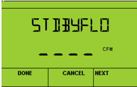
Standby flow setpoint in CFM [nciStbyMinFlowSetpt]
