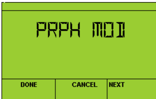
Configure modulating periph heat [nciLogicalOutVav, PrphHtgMod]
