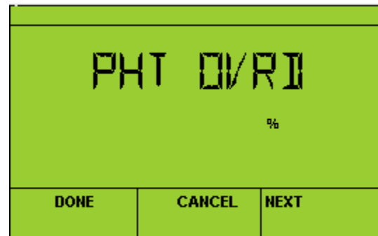
Peripheral Heat override as a percent number of stages or modulation [nviValveOvr, periphPos]
