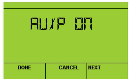
Configure Auxiliary Relay pulse ON [nciLogicalOutVav, AuxPlsOn]
