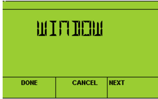
Configure window sensor [nciLogicalInVav, WindowOpen]
