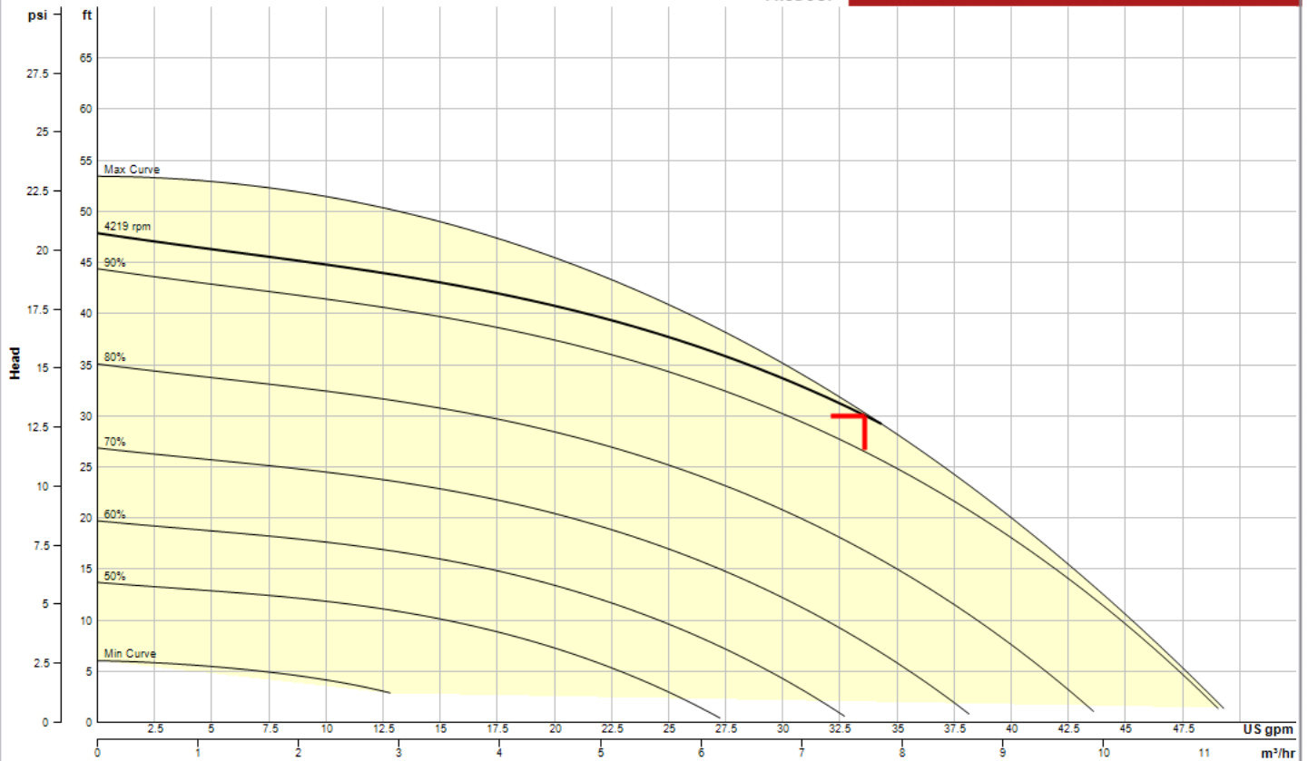
Performance curve meets 14.6 / ISO 9906 acceptance criteria
