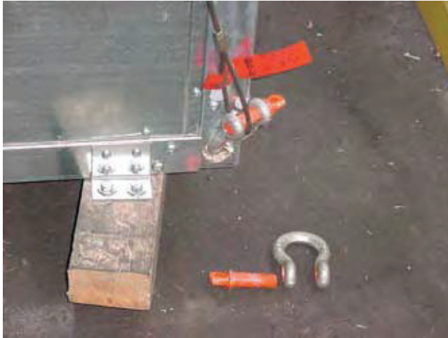
FIG. 1-4 – PROPER LIFTING WITH SHACKLE AT CORNER
