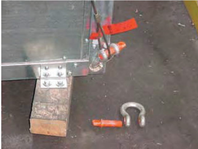
FIG. 1-4 – PROPER LIFTING WITH SHACKLE AT CORNER
