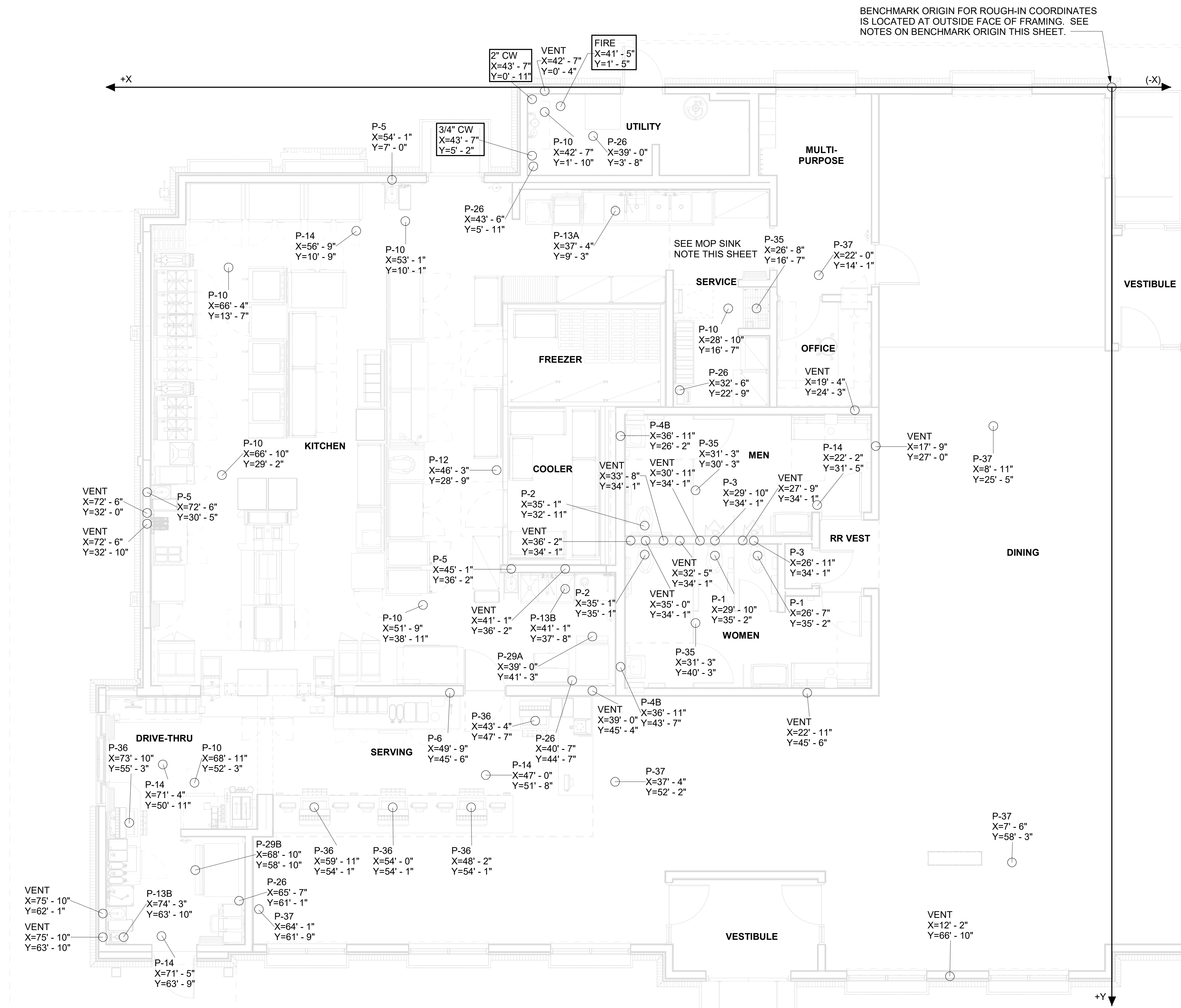
1 SLAB ROUGH-IN PLAN 1/4" = 1'-0"
