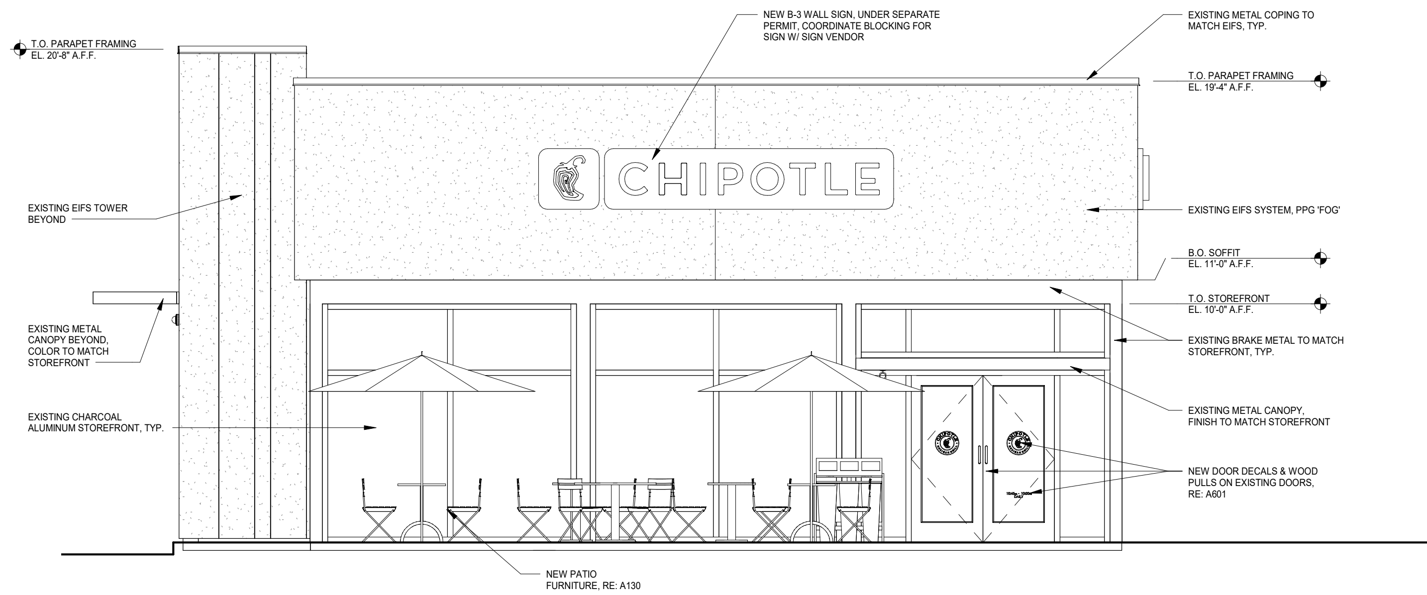
4 BUILDING ELEVATION - NORTH 1/4" = 1'-0"
