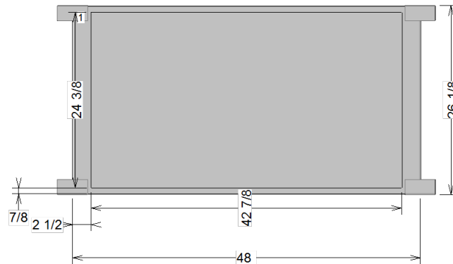
Detailed Elevation View: Back - Measurements in inches
