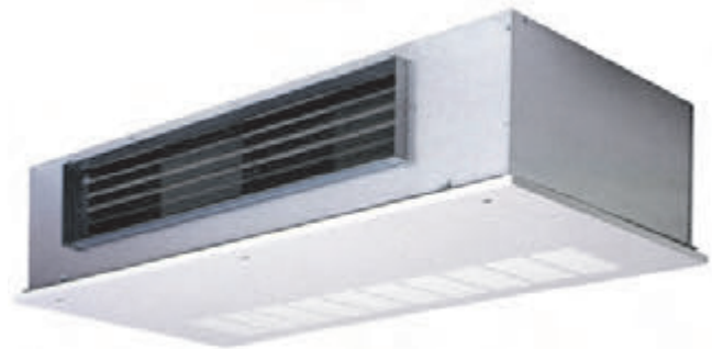
42CK Cabinet model with telescoping flip-down panel and stamped louver bottom return or duct collar rear return. (200-1200 cfm)
