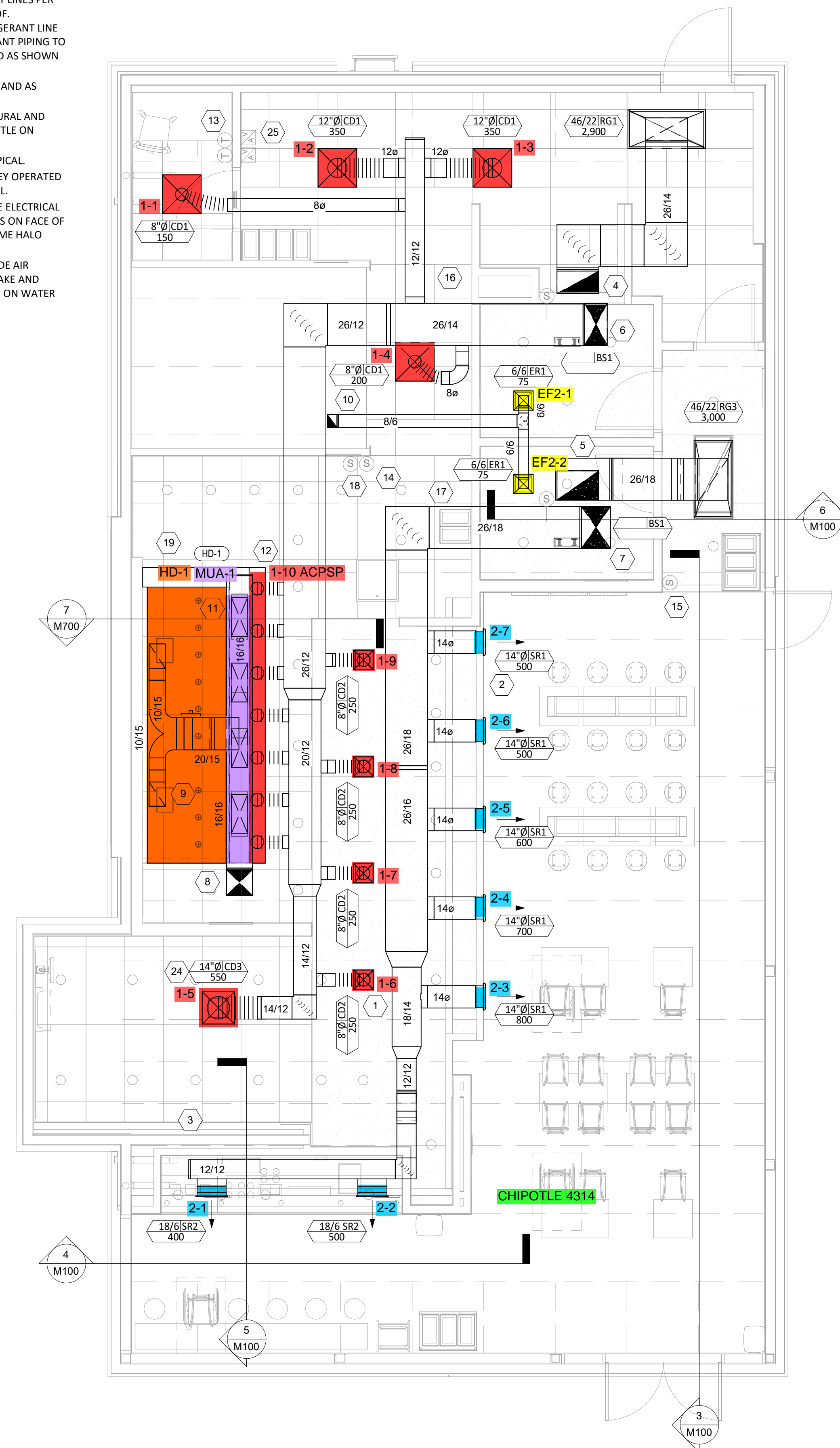
1 M100 1/4" = 1'-0" HVAC FLOOR PLAN
