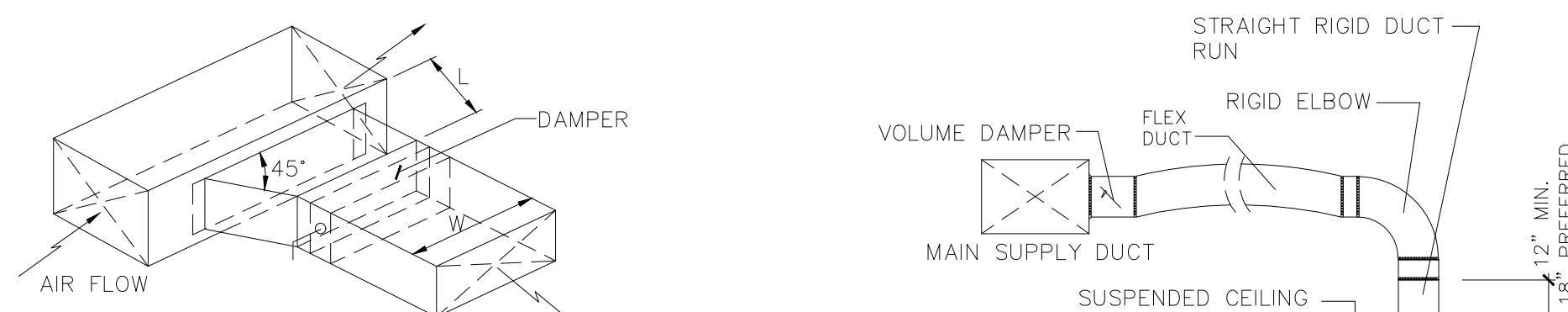
BRANCH DUCT TAKEOFF DETAILS N.T.S.
