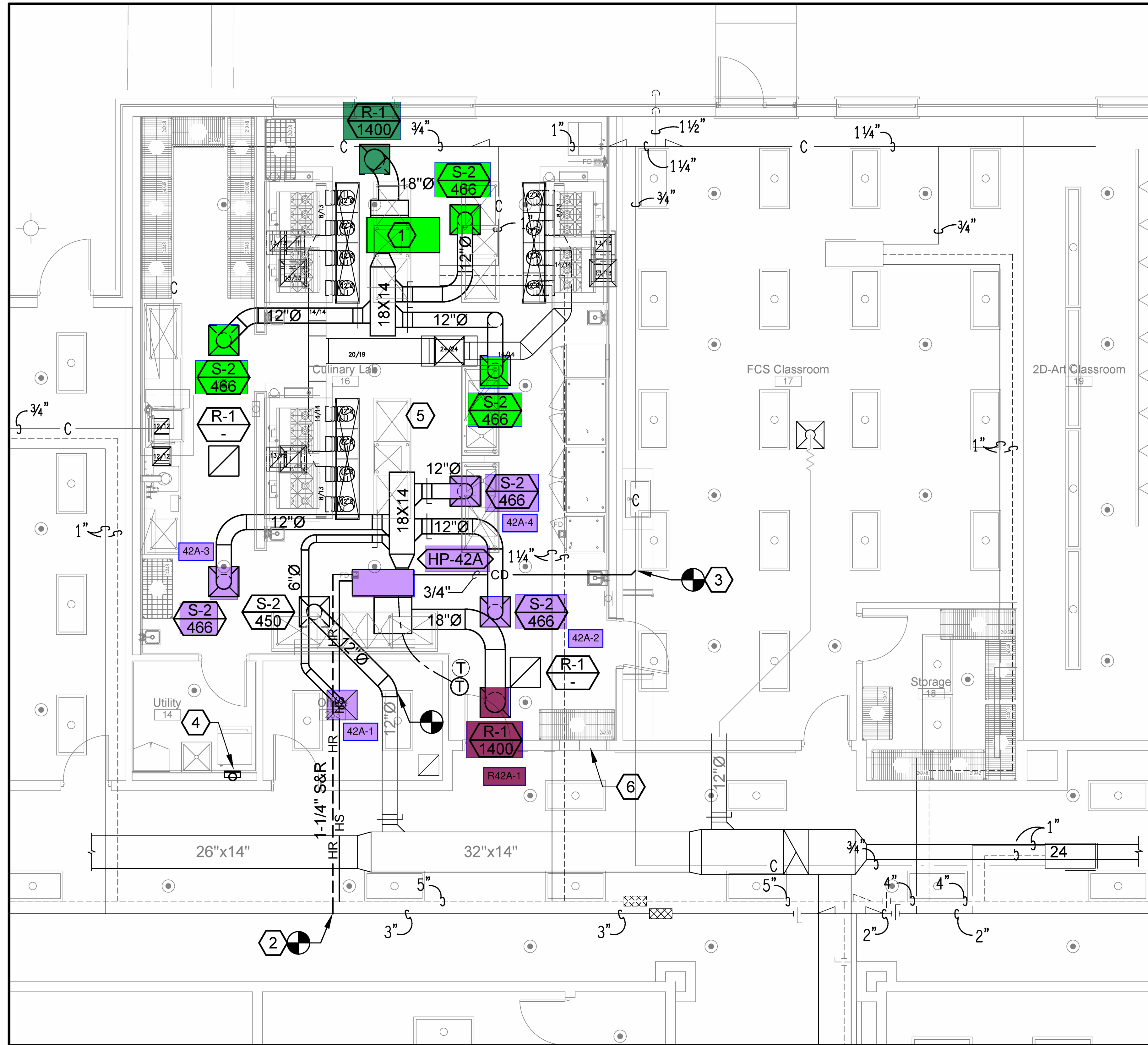
1 PARTIAL MAIN LEVEL FLOOR PLAN - MECHANICAL - HVAC SCALE: 1/4"=1'-0"
