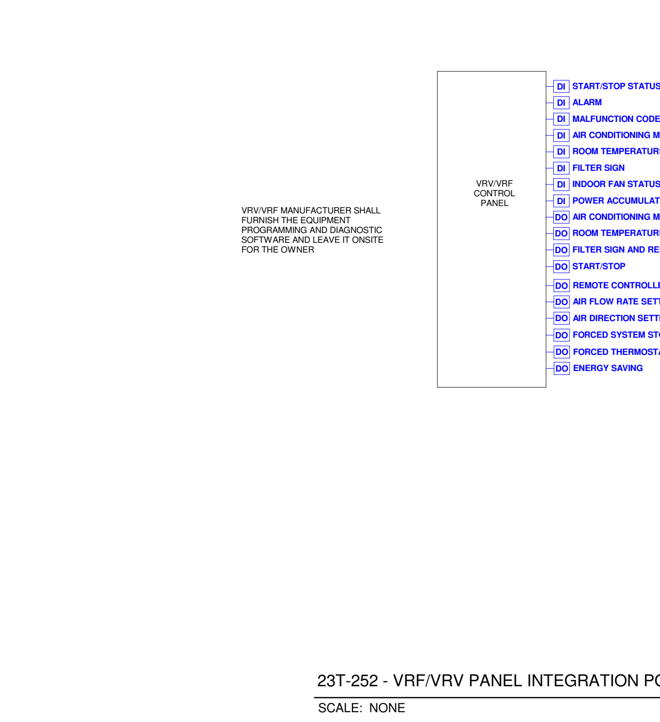
231-252 - VRF/VRV PANEL INTEGRATION POINTS SCALE: NONE
