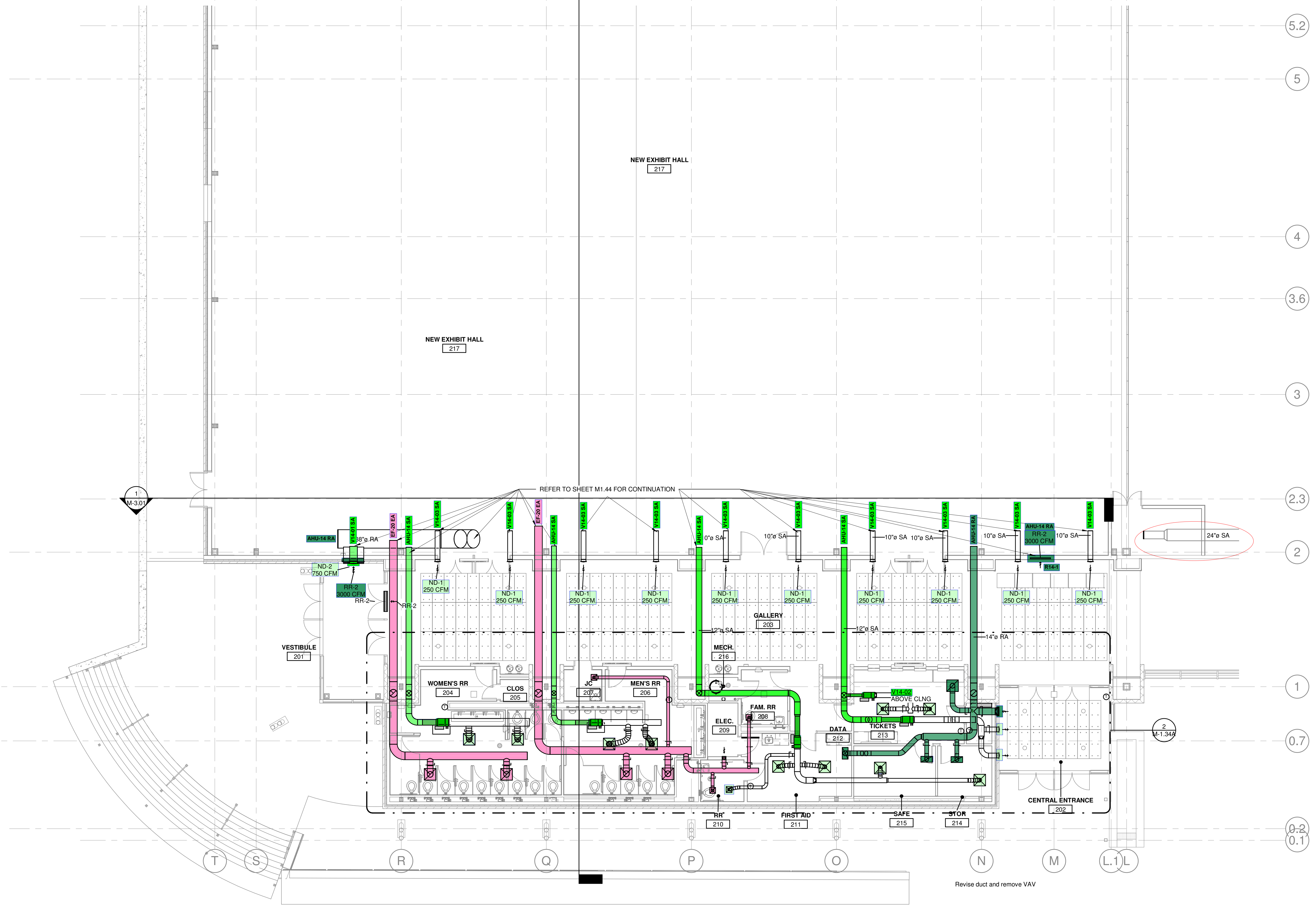
1 MECHANICAL DUCTWORK SECOND LEVEL PLAN - 4A M-1.34A 1/8" = 1'-0"
