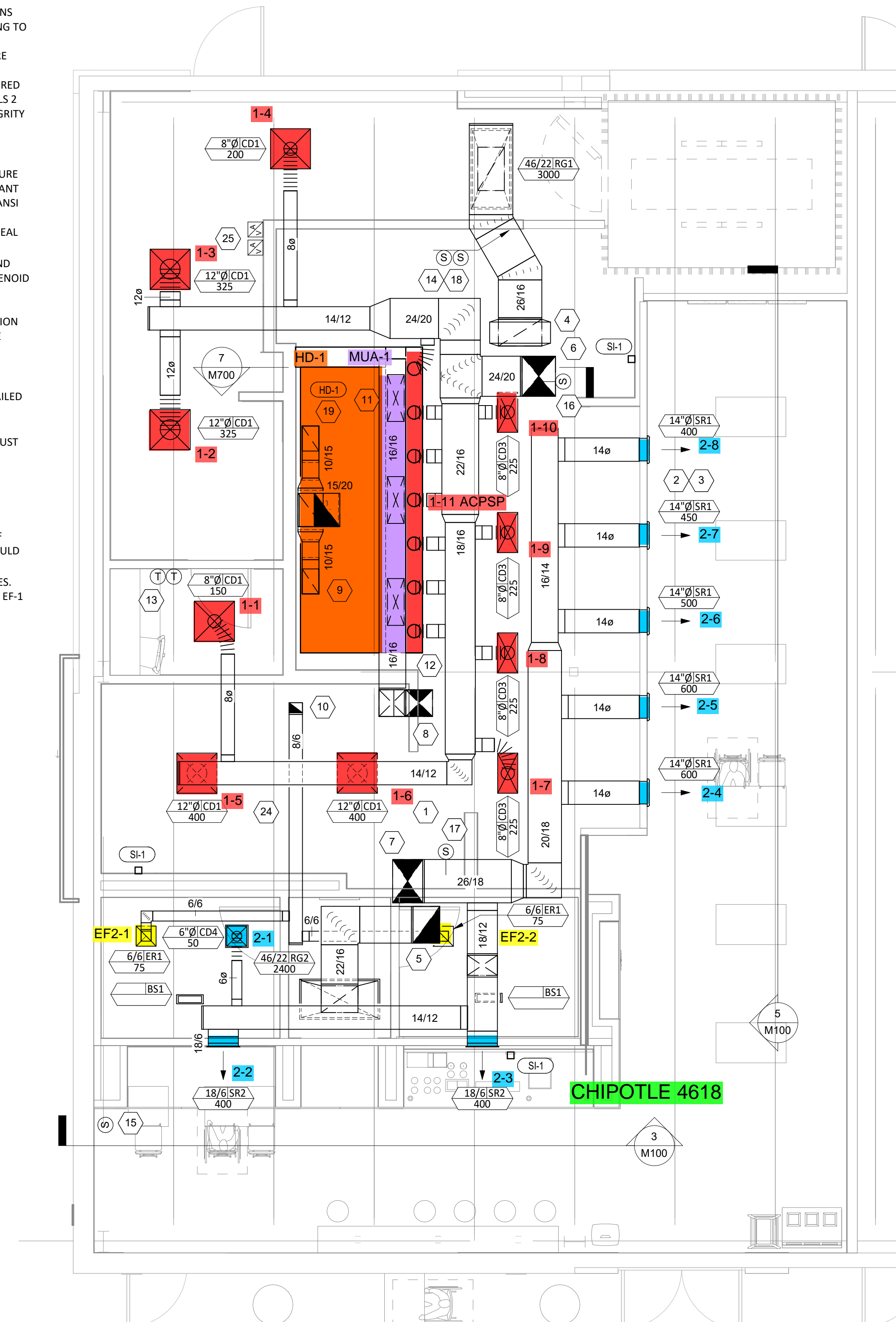
1 HVAC FLOOR PLAN 1/4" = 1'-0"
