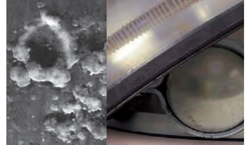
Prevent EDM Pitting and Fluting Damage
