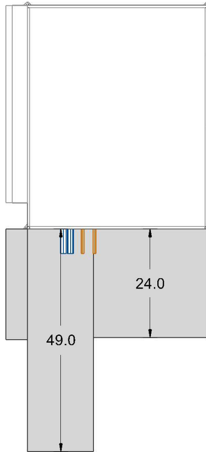
PLAN VIEW - SERVICE CLEARANCE
