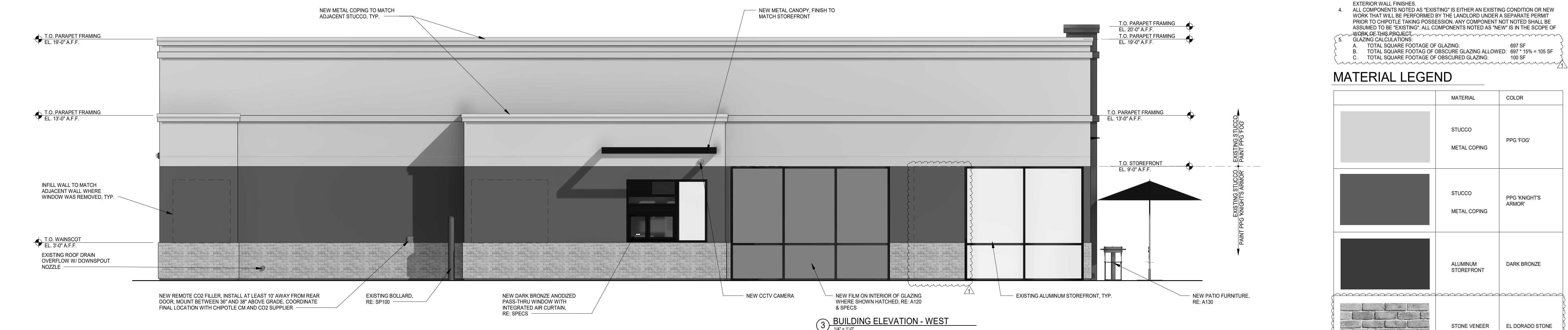
3 BUILDING ELEVATION - WEST 1/4" = 1'-0"
